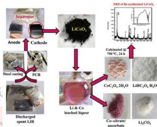
Fig. 1. Photographs of the LIB after dismantling & products before and after selective precipitation.
