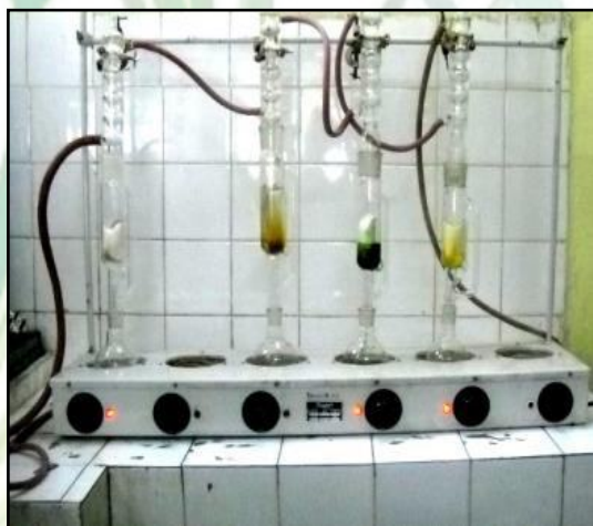
Fig. 4: Soxhlet apparatus for extraction.
